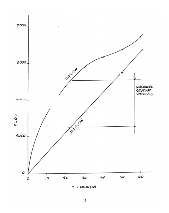
Select 20' x 40' x 3.0' deep pond with 3:1 side slopes for maintenance. Allow 1.0' freeboard except an emergency spillway, where 0.5' freeboard is to be used.
