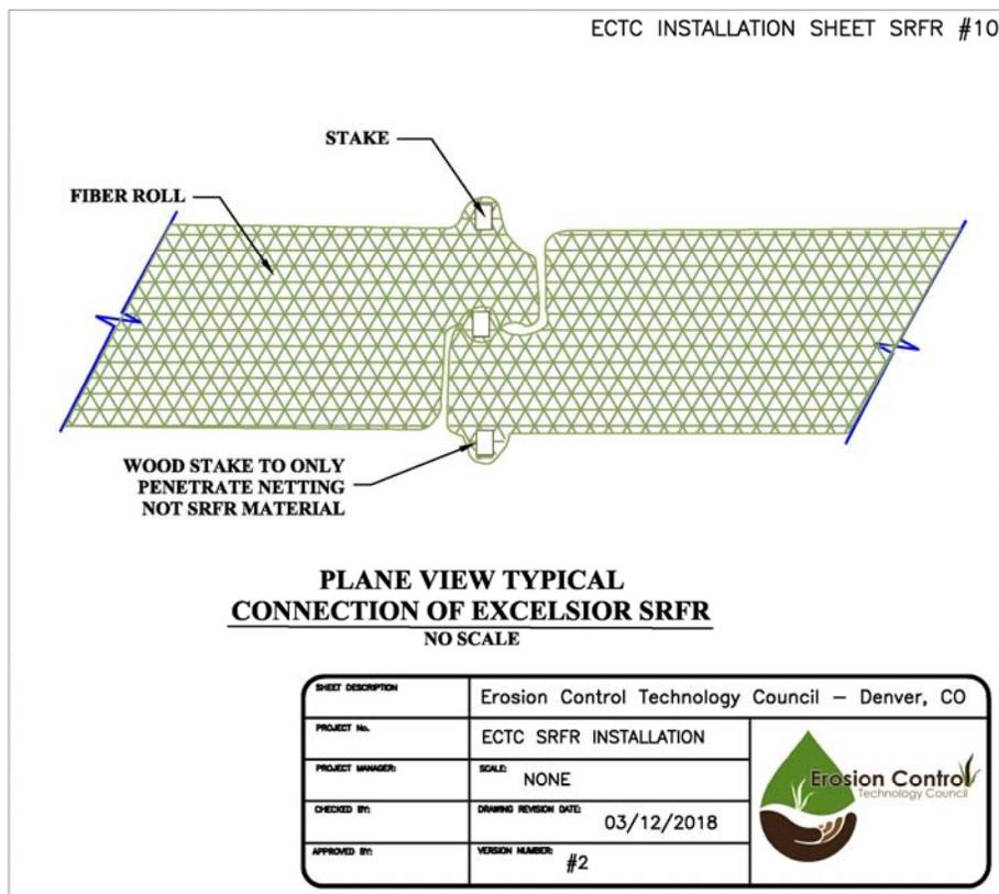
Figure 10. Typical connection of a wood SRFR.
