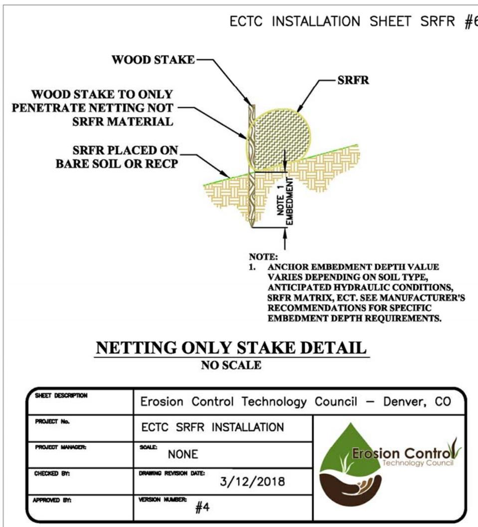
Figure 6. Stake through netting only on soil.
