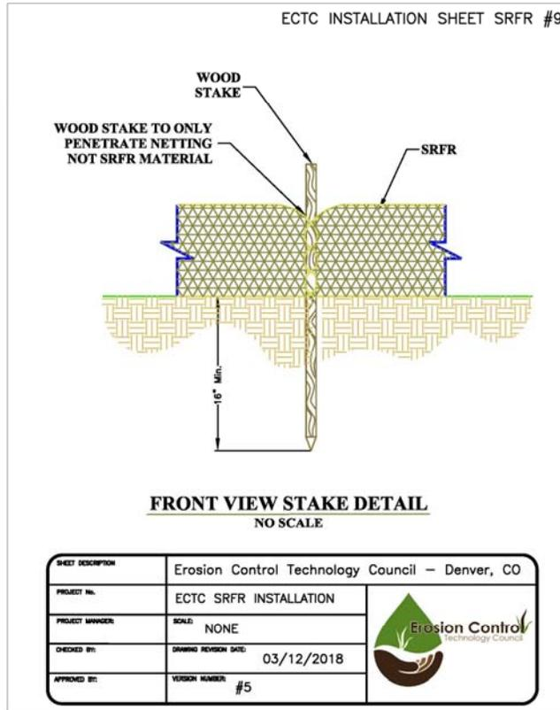
Figure 9. Abutting SRFRs with a common stake.
