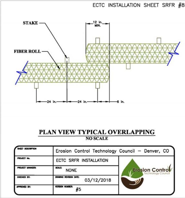
Figure 8. Overlapping SRFRs with laced stakes.
