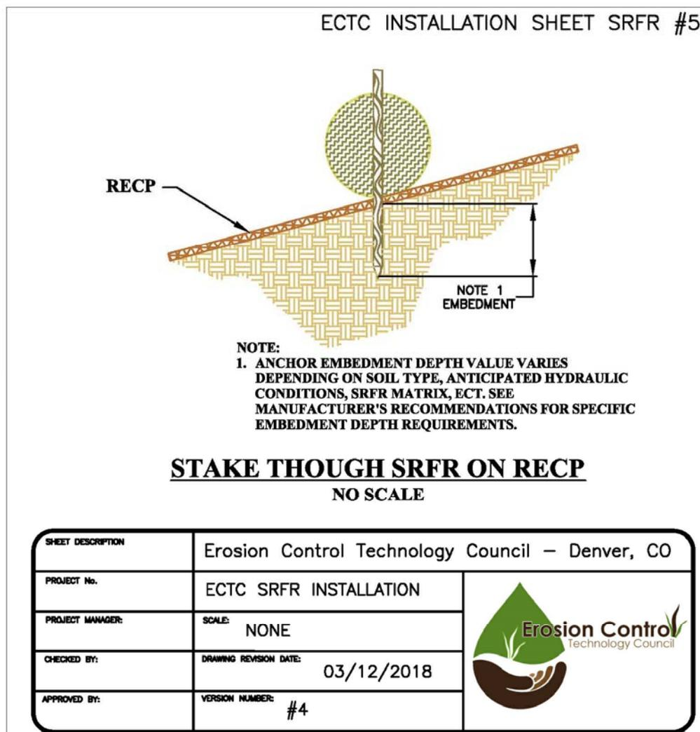
Figure 5 Stake through RECIP on top of RECIP/HECP.
