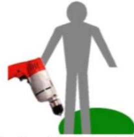
A metallic part in contact with an energized wire while the person is also in contact with the ground.
