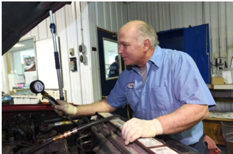
Technician Les Smith uses a pressure gauge to measure fuel pressure at Brown’s Auto Service March 6, 2017
