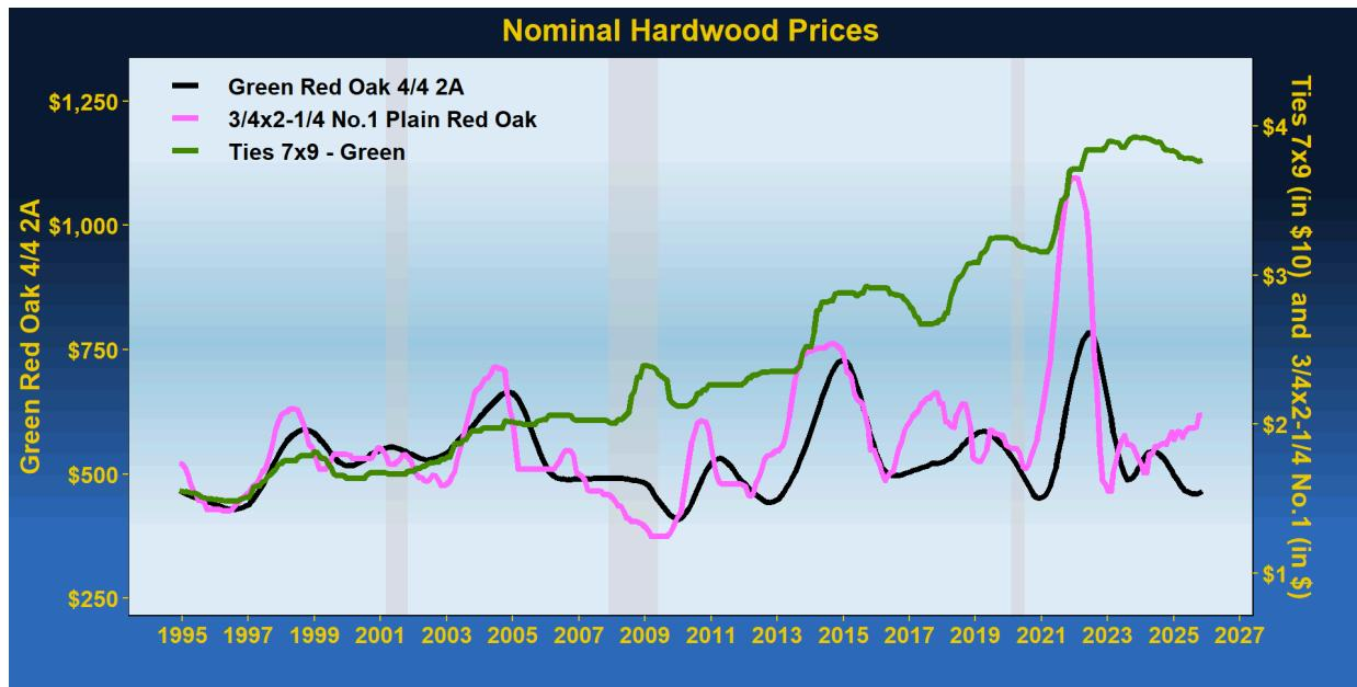
Note about the right side Y-axes: The "Ties 7x9 - Green" and 3/4x2-1/4"No.1 Plain Red Oak are on the same axis. In order to show the relationship of the various wood product prices, the price of the "Ties 7x9 - Green" is scaled down by 10. Thus, the right Y-axes for the Ties should be read as 10 multiple.
