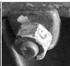
Close-up of lug nut holding rim to wheel.
