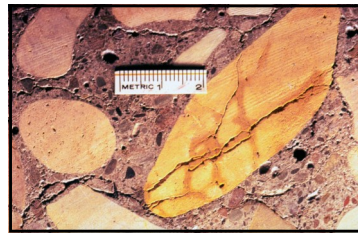
Non Air Entrained Concrete breaking up from the inside out
