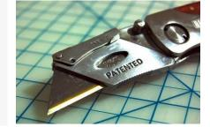
There have been cases where workers have suffered injuries from exposed blade tips. This is because the blades did not completely retract into the handle. That's why it's important for workers to use the proper size blades or replace defective retraction mechanisms. Some companies use self-retracting utility knives – the blade automatically retracts when not in use. The following are safety precautions to keep in mind when using utility knives:
