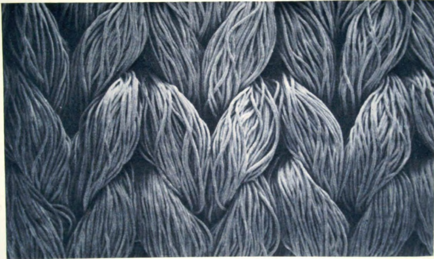
Figure 28-2. SEM of outer surface of DeBakey standard knit Dacron vascular prosthesis ( \times 37 ).
