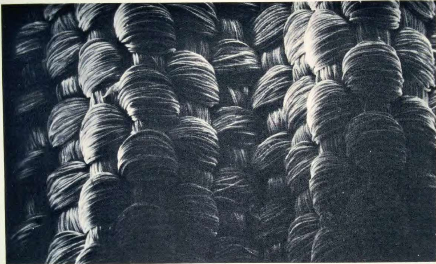
Figure 28-1. Scanning electron micrograph (SEM) of outer surface of DeBakey woven Dacron vascular prostheses ( \times 37 ).
