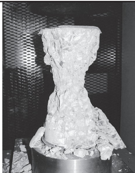
Fractured Test Specimen at Failure
