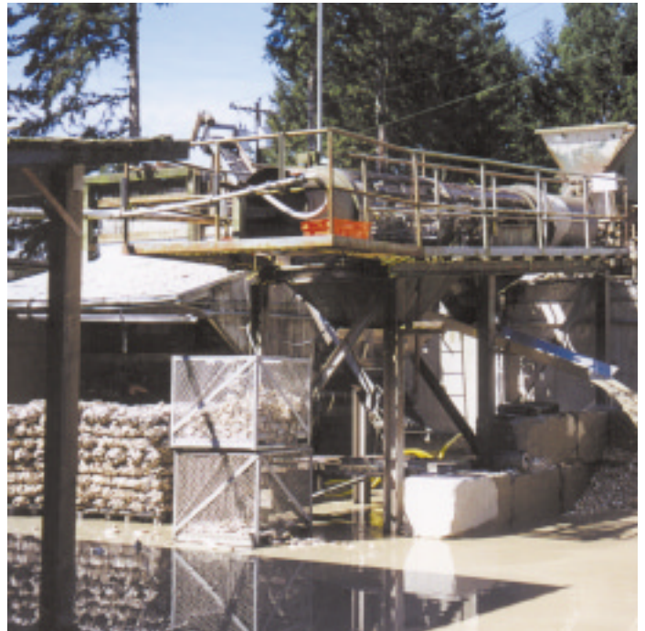
Oyster shells, a by-product of the oyster shucking process, are reused by aging, washing and bagging for “cultch,” to which seed oysters will attach.
