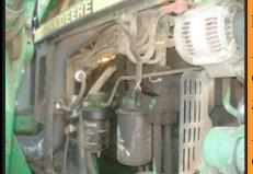
A pressure washer should be used to remove all caked-on grease, oil, and crop residue. A clean engine will run cooler, operate more efficiently, and greatly reduce your chance for fire.
