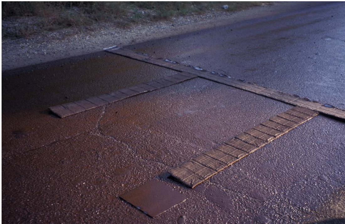
Figure 7. ASTM D2995 Method A pads following tack coat application.
