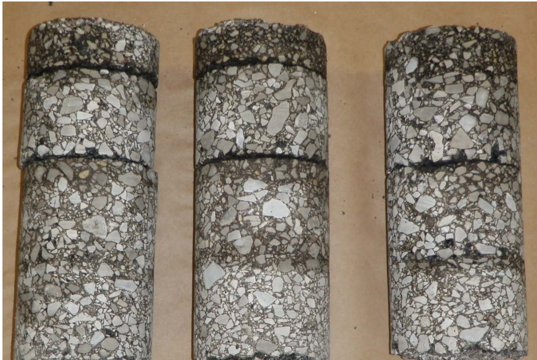
Figure 3. Cores showing layer debonding from Missouri.
