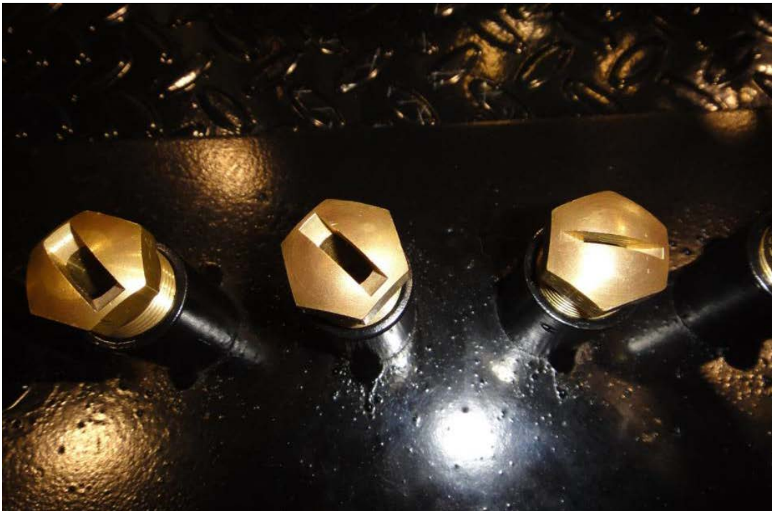
Figure 8: Examples of different nozzle sizes for different application rates.
