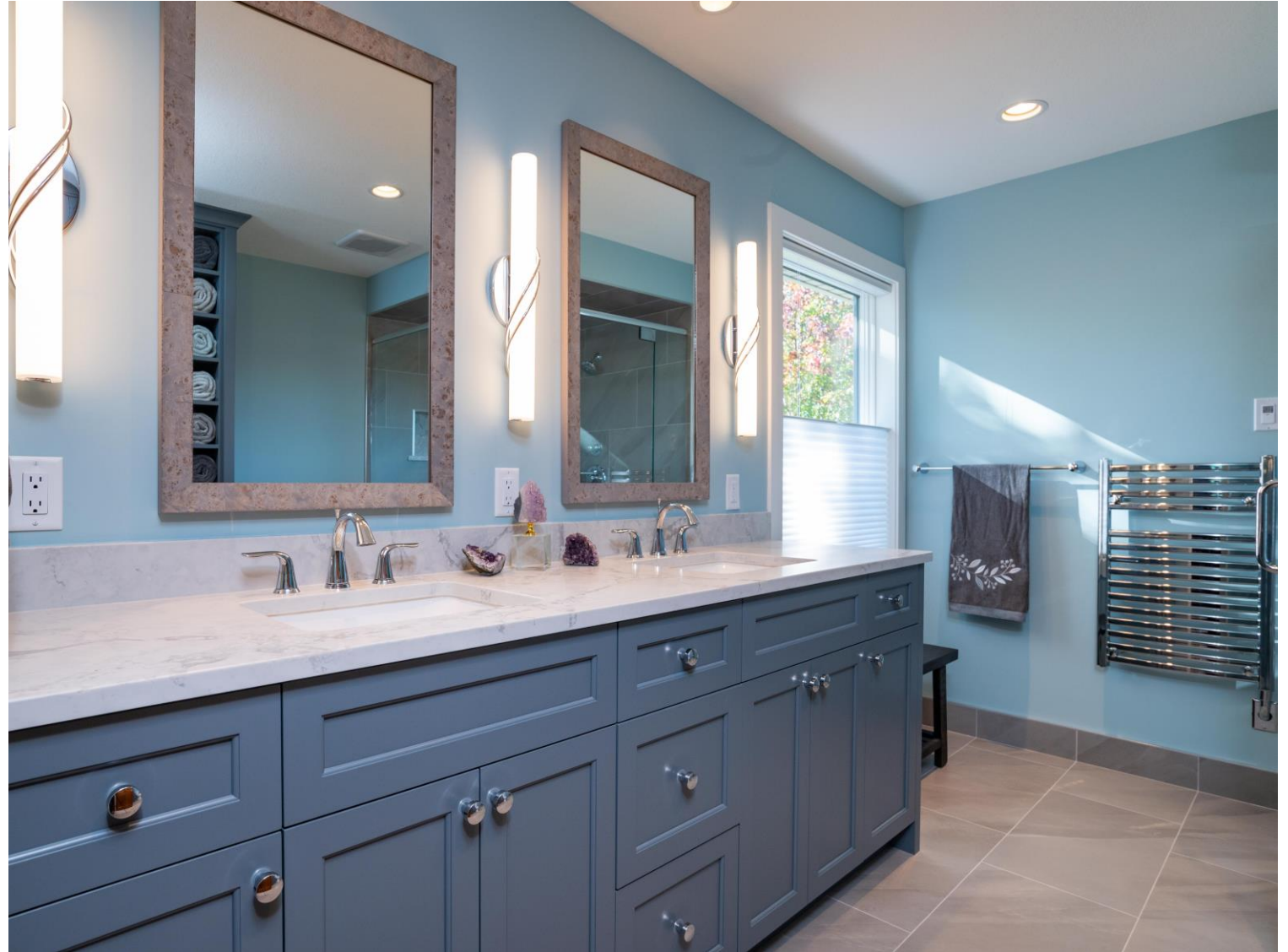
Frameless vanity cabinet has flat panel doors with a bead and a Carrara Gaviota quartz top. The framed mirrors are perfectly centered between 3 dimmable Hinkley vanity lights.
