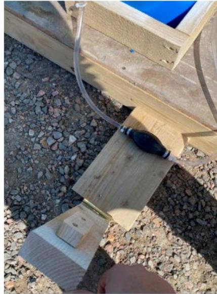
Bulb placement under foot pump assembly.
