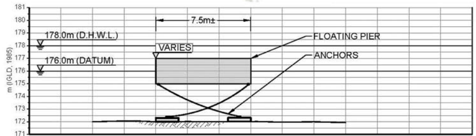
Figure 3.3: Typical Floating Pier Cross Section
