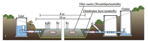
Fig. 1. Conceptual diagram of subsurface flow constructed wetlands (SSF-CWs) with horizontal flow including inlet well, distributions pipes, distribution layer (seashells), filter matrix (willow
