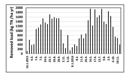
Fig. 1. Removal of TN load in a vegetated drainage ditch during the period 16.1.2015 – 8.12.2016.
