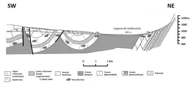
Fig. 2. Cross-section of the hydrogeological system.
