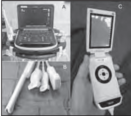
Figure 2. A. A laptop sized portable ultrasound system. B. Differing ultrasound transducers from left to right, a 7 MHz endocavitary transducer, a 3 MHz small curvilinear transducer, a 5 MHz wide curvilinear transducer. C. Handheld ultrasound machine.
