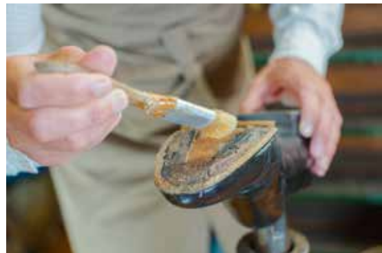
Fig. 24: Adhesive bonding technology in shoe repair 37
