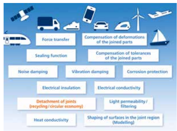
Fig. 4: Possible functions of an adhesive in an adhesively bonded joint
