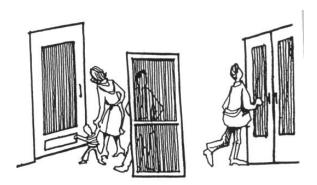
Many original doors have been replaced by standard aluminum and glass commercial doors. Although lacking in historical character, they are generally unobtrusive. Aluminum doors and storefronts can be made more compatible by painting them a dark color. An exposed aluminum surface must be cleaned and prepared for a zinc chromate primer or metal primer, followed by appropriate finish coats. New aluminum should be exposed to weather for at least two months before painting.
