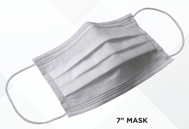
7" medical mask with elastic earloops. Outer and inner layers composed of spunbond polypropylene. Middle layer is meltblown polypropylene. Binding ties tensile strength  $\geq$  10N, ventilation resistance  $\leq$  49Pa/cm2, bacterial filtration efficiency  $\geq$  95%. Available in White.
